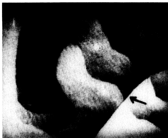
FIG. 10. Brewster-angle microscopy image with analyzer of a sodium myristate film at bulk concentration 6 mg/l. An example of the deformations of the defect lines that occur during a few minutes when the dense domains, very close to each other, are distorted by their neighbors because of strong repulsive dipolar interactions. The bar represents 50 \mu\text{m} . The arrows indicate the juncture between the neighboring domains.
